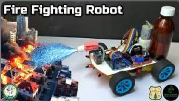
**Concept:** A multi-purpose robot that follows a line to reach a "fire zone," picks objects or pushes obstacles, and extinguishes a small LED-based fire.
