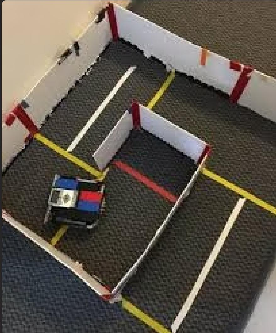
**Concept:** A robot that detects walls using ultrasonic sensors and finds its way out.
